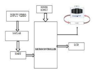
Transmitter is the electronic device to transmit the data to the receiver, the video is given as a input to the MATLAB section, the controller which receive the data send a serial port using UART communication protocol, these data is send to the receiver part.
